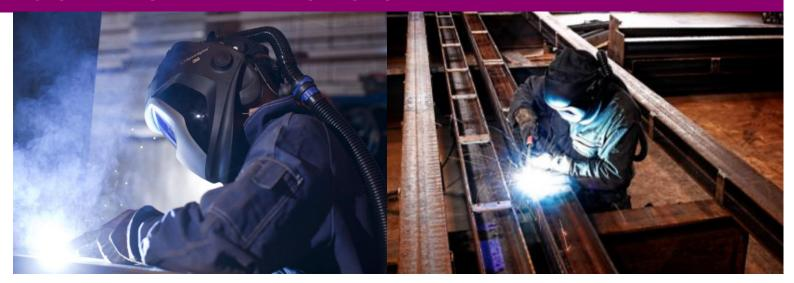
On-gun and local extractors remove much, but not all, of the welding fumes right at the source, thereby reducing their spread to other areas. Well-designed general ventilation will remove welding fumes that were not immediately captured at the workstation and exchange them with fresh air.
